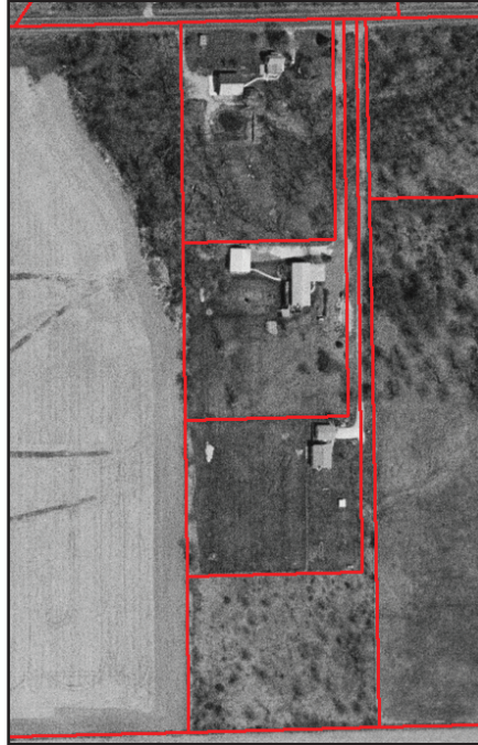
Image 3: Example of a flag lot in Tazewell County. In this image, three flag lots are stacked together, creating access problems and inhibiting future land subdivision.
